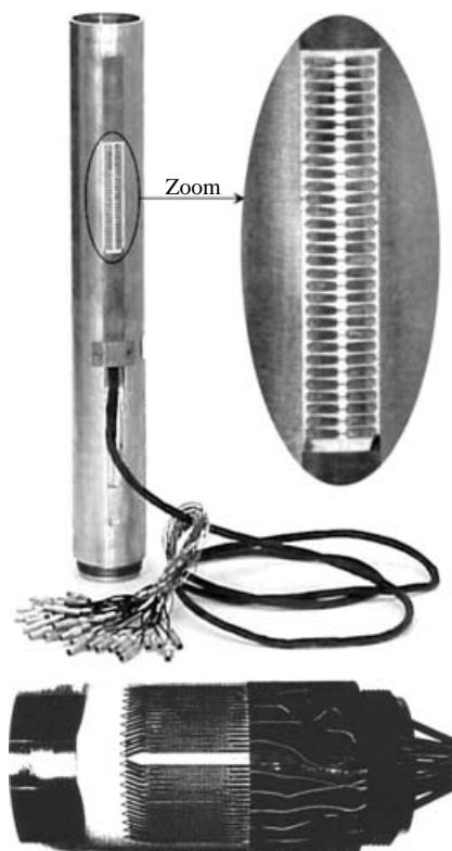
FIGURE 4. Instrumented model segments for both axial and circumferential heat transfer array measurement. In the axial array the thin-film sensors comprise the fine central line; the thicker outboard lines are low resistance gold paint connectors. For the circumferential array, the platinum sensor is the V-shape.
